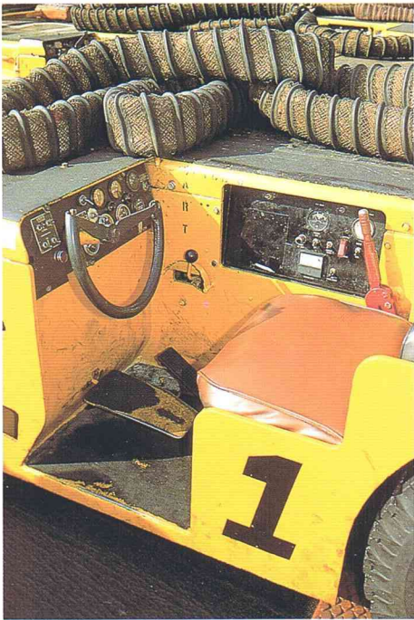
Fig.4 Ample space for the mule driver with monitoring panel in front and turbine operating panel on the right hand side. Note the structure of the hose on top.
