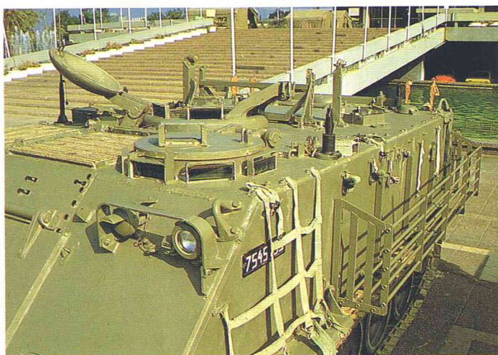
Fig.4 Upper left front of the real CCV. Pay close attention to the smaller details which make the whole picture. Note how the tie-down straps are fitted and the single headlight, also the white on black registration plate partially covered by the forward straps. These embossed ID plates are designed to withstand a destructive fire which would certainly burn off painted-on numbers, making identification of a knocked-out vehicle very difficult. Two are usually carried, one on each side of the vehicle.
