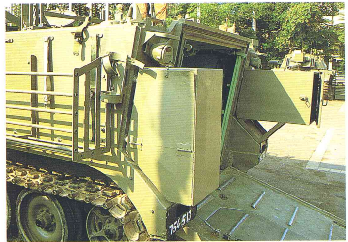
Fig.5 Note the unusual shapes of the storage boxes and how they are mounted to the vehicle's rear end. The registration number is repeated on the left rear mudguard. ID plates in this location are painted instead.
