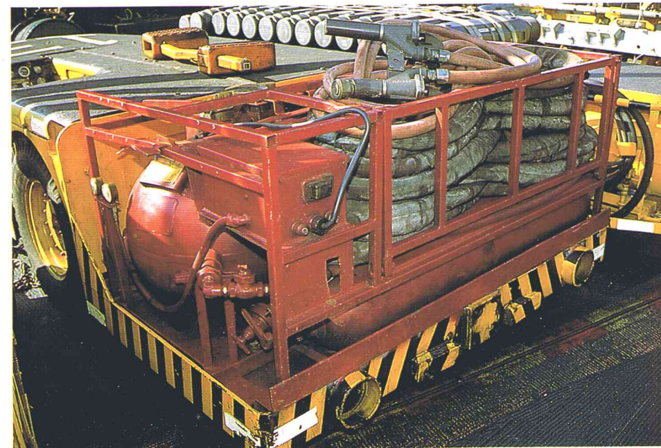
Fig.10 Close view on the valves, pressure gages and spherical pressure unit. Note the dual spray-nozzles on top of the hoses and the deletion of the tow pintle at the rear.
