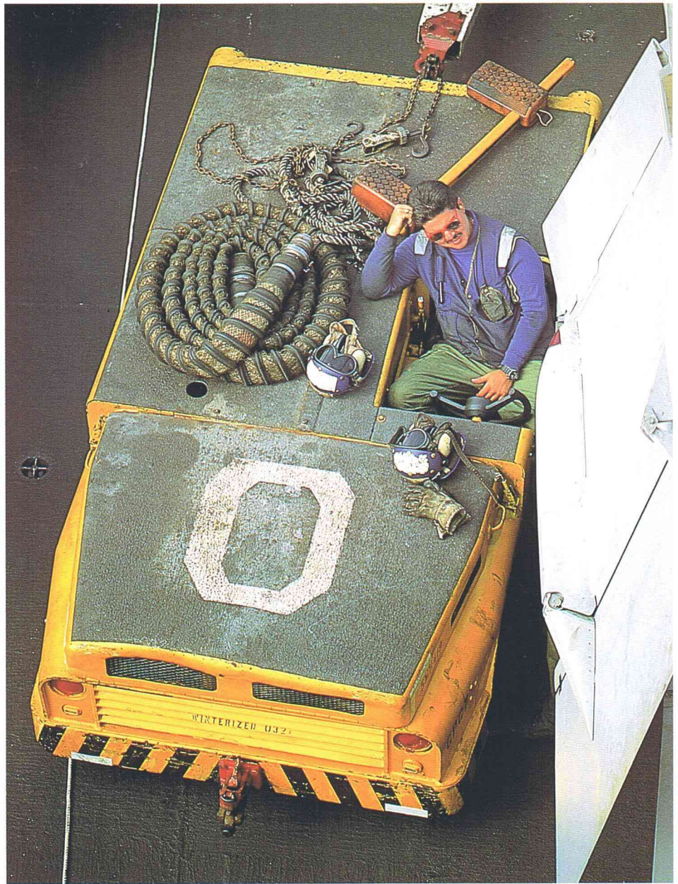
Fig.4 Ample space for the mule driver with monitoring panel in front and turbine operating panel on the right hand side. Note the structure of the hose on top.
